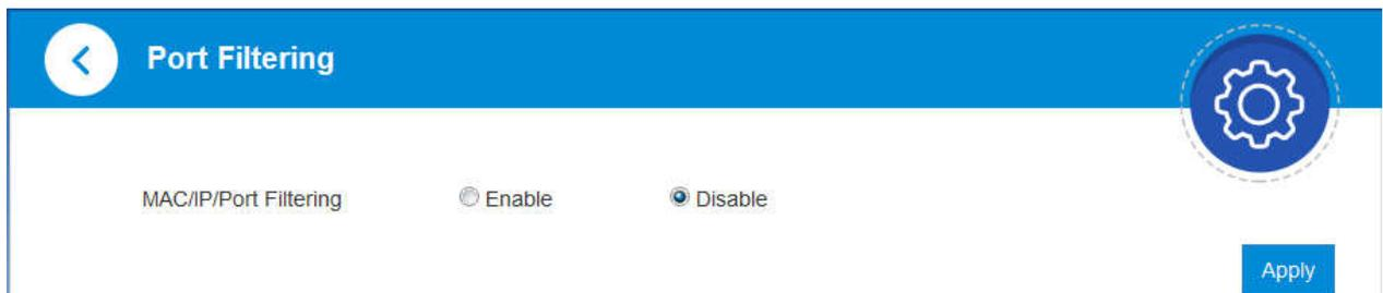
2. Set **MAC/IP/Port Filtering** to **Enable**, **Default Policy** to **Accepted** or **Dropped** and click **Apply**, the filter settings will appear as shown below:
