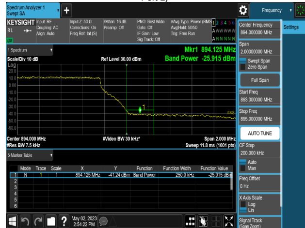
Plot 8-394. Band Edge Emission Summary Data Plot (MSR 3C_NR n5_2C_10M+10M+LTE B5_1C_5M_QPSK - High Channel_4T, Port 2)
