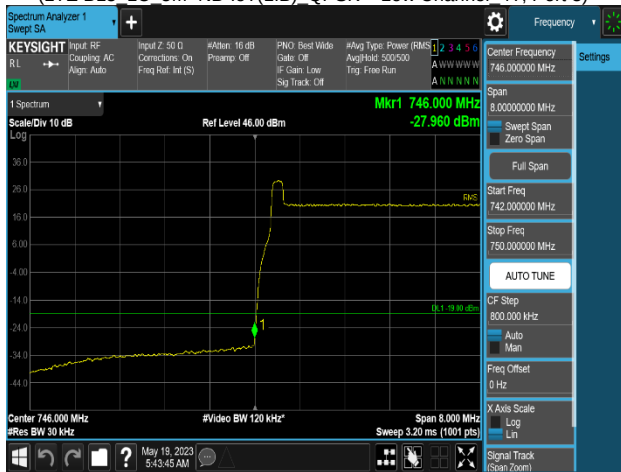
Plot 8-417. Band Edge Emission Summary Data Plot (LTE B13 1C 10M+NB-IoT(2GB) QPSK - Low Channel 4T, Port 3)
