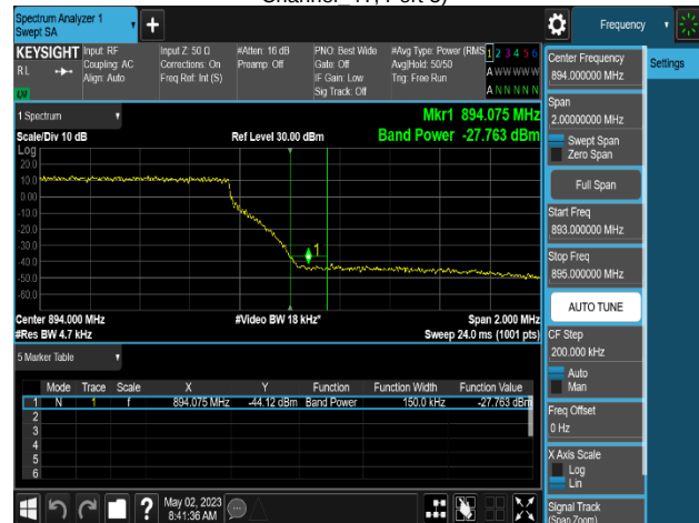
Plot 8-390. Band Edge Emission Summary Data Plot (MSR 2NC_DSS B(n)5_1C_10M+LTE B5_1C_5M_QPSK - High Channel 4T, Port 2)
