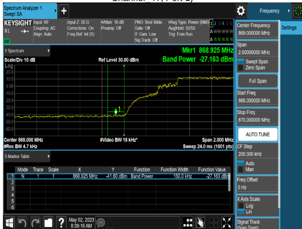
Plot 8-389. Band Edge Emission Summary Data Plot (MSR 2NC_DSS B(n)5_1C_10M+LTE B5_1C_5M_QPSK - Low Channel 4T, Port 0)
