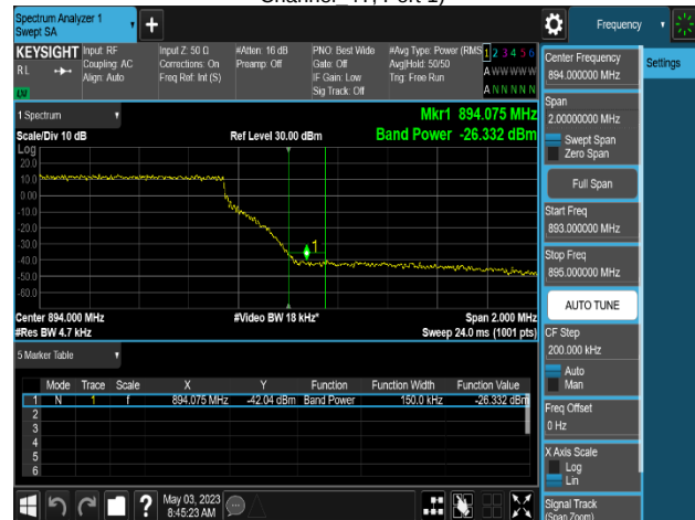
Plot 8-402. Band Edge Emission Summary Data Plot (MSR 2NC_DSS B(n)5_1C_10M+NR n5_1C_5M_QPSK - High Channel 4T, Port 2)
