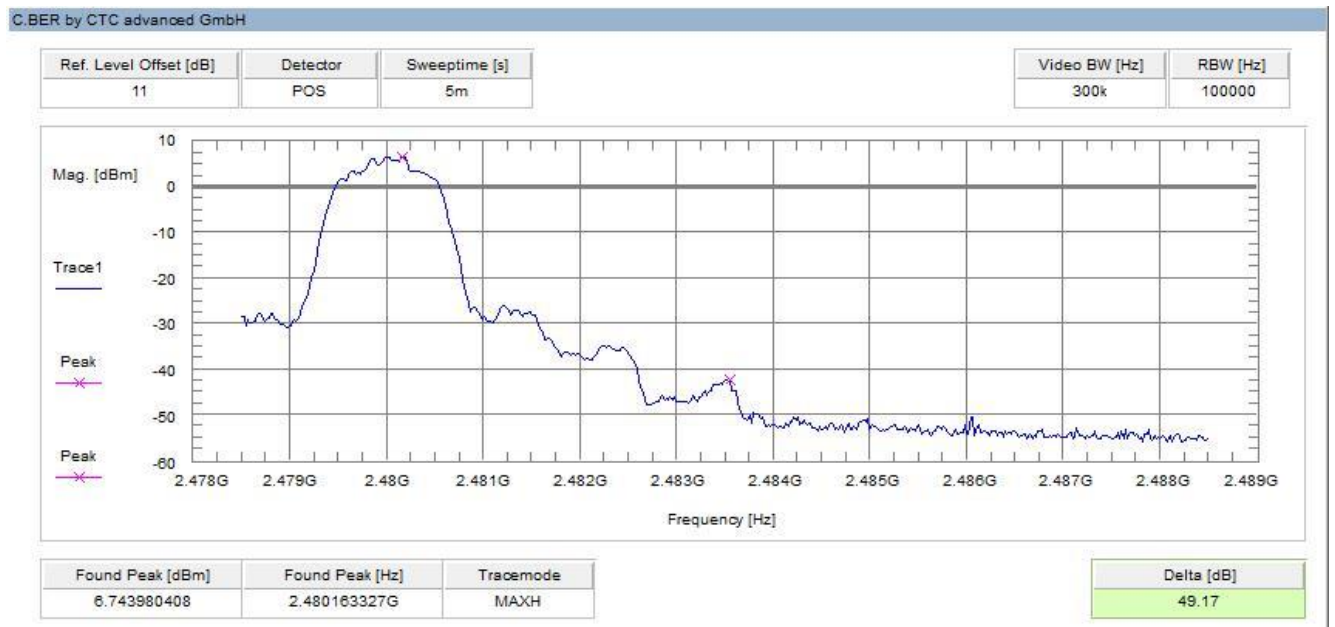
Plot 8: Upper band edge – hopping off, Pi/4 DQPSK modulation
