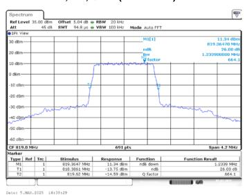
LTE band 26, 1.4MHz Bandwidth, MID, 16QAM (-26dBc BW)
