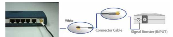
3) After you have connected the signal booster to the certified wireless router, take the antenna included in the package and connect it to the antenna connector on the signal booster. Screw the antenna base in clockwise until the antenna is firmly connected to the booster.
