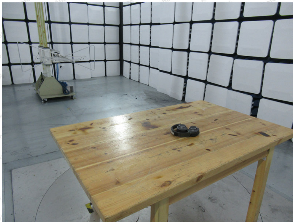
Photo of Radiation Emission Test
