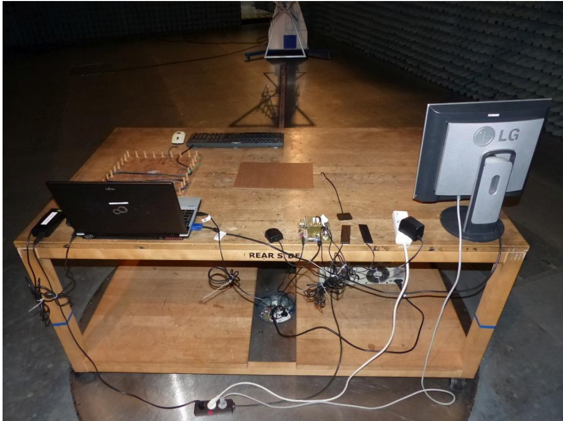
Photo 2: Test setup AE02 for radiated measurements, unintentional radiator §15) single device setup, computer peripheral.
