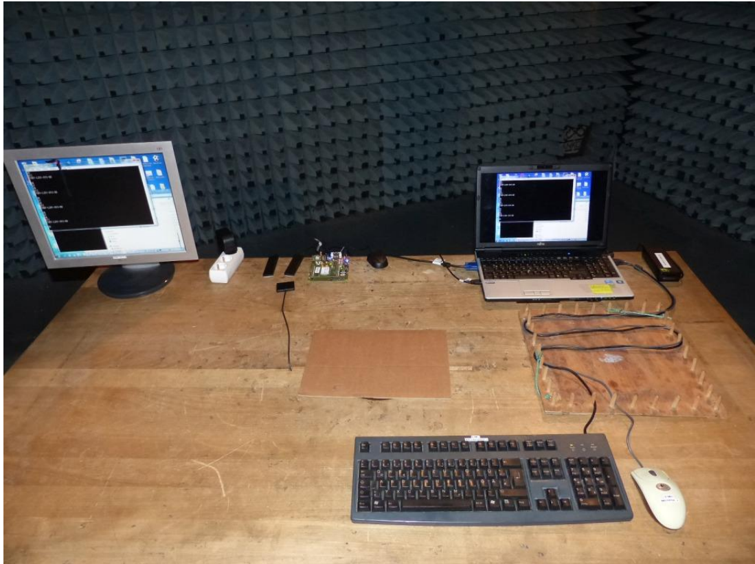
Photo 1: Test setup AE02 for radiated measurements unintentional radiator §15) Single device setup, computer peripheral.
