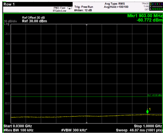
Channel: MIDDLE, Modulation: 64QAM, BW=5MHz, Range: 30MHz - 1GHz
