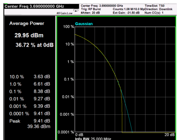
Channel: TOP, Modulation: 16QAM, BW=20MHz, CCDF
