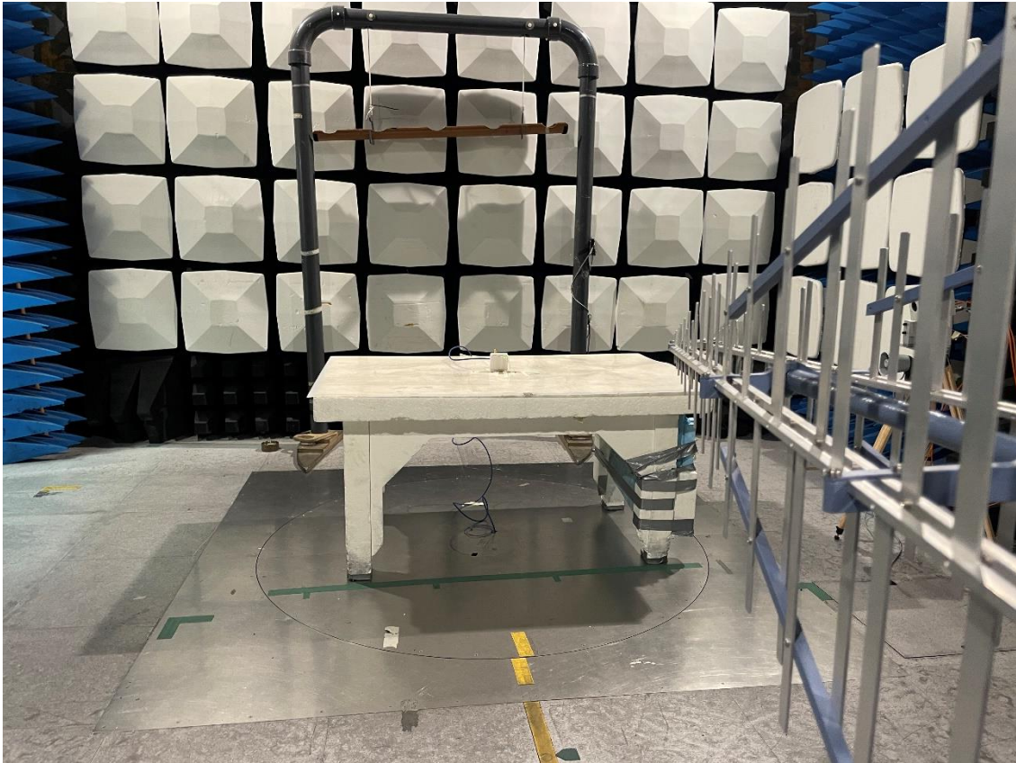
Photo of the test set-up for radiated emission 30 – 1000 MHz
