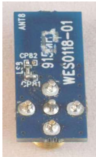
Figure 108. Small Sized Printed ILA Antenna
