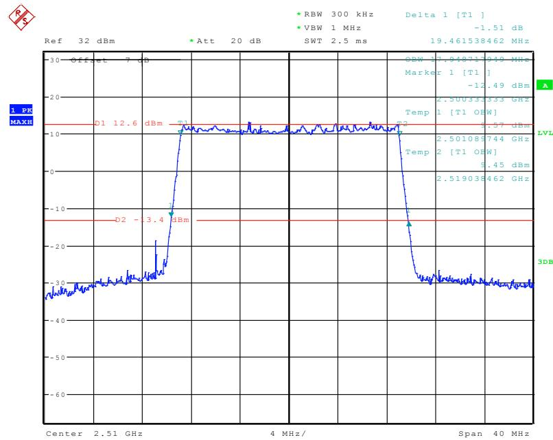
**16-QAM (20.0 MHz) - 26 dB Bandwidth & 99% Occupied Bandwidth, Low channel**
