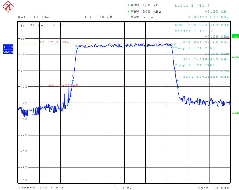
**16-QAM (5.0 MHz) - 26 dB Bandwidth & 99% Occupied Bandwidth, High channel**
