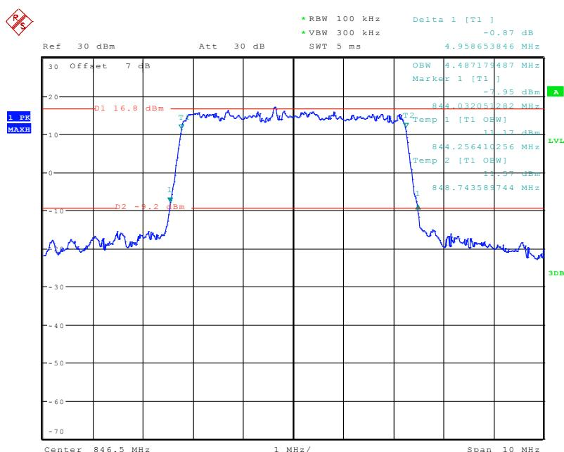
**QPSK (10.0 MHz) - 26 dB Bandwidth & 99% Occupied Bandwidth, High channel**
