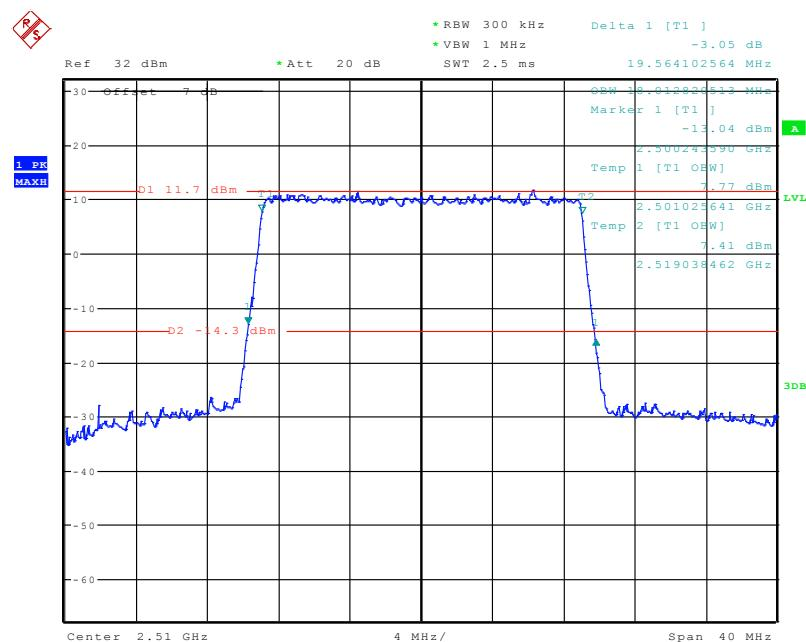
**QPSK (5.0 MHz) - 26 dB Bandwidth & 99% Occupied Bandwidth, Middle channel**
