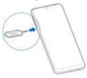
2. Pull out the card tray and place the nano-SIM card(s) and the microSDXC card on the trav. as shown. Carefully slide the tray back into place.
