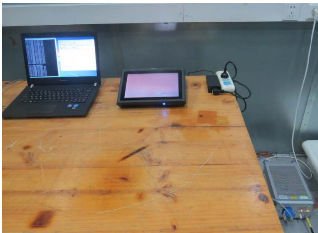
Picture 2 Conducted Emission Test Setup
