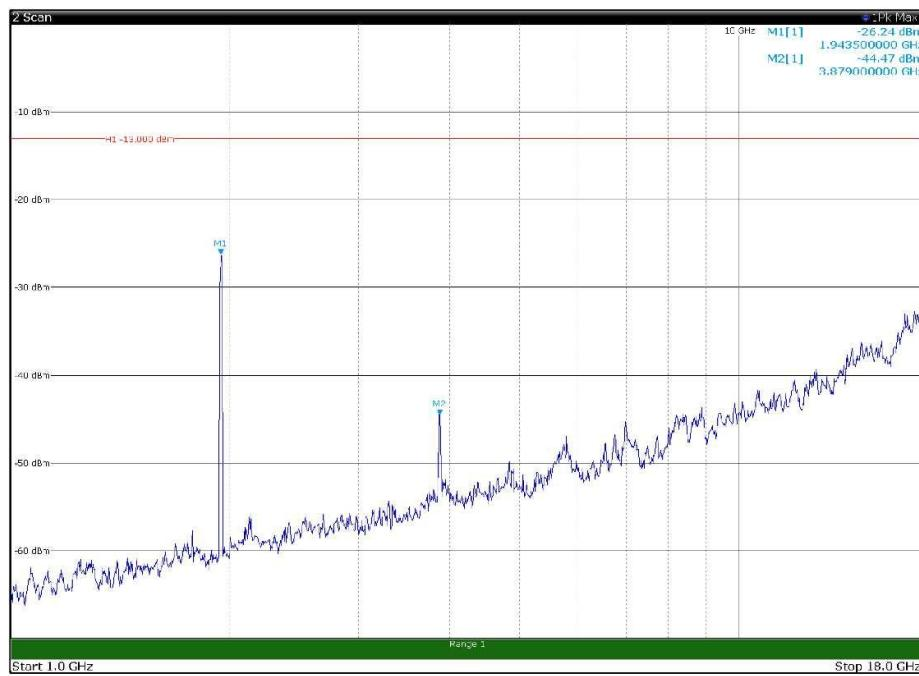
Channel: BOTTOM, Modulation: 64QAM,
