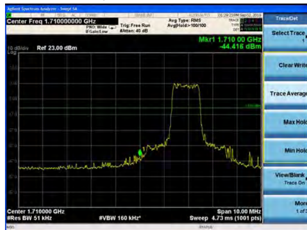
LTE Band 66 QPSK 20MHz CH-Low, 100%RB
