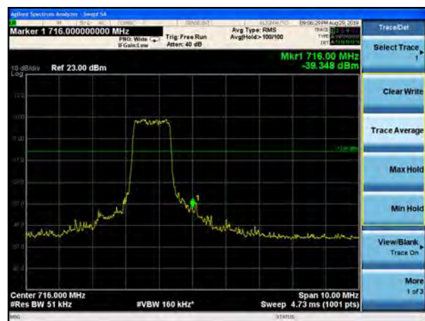
LTE Band 85 16QAM 5MHz CH-High, 1 RB
