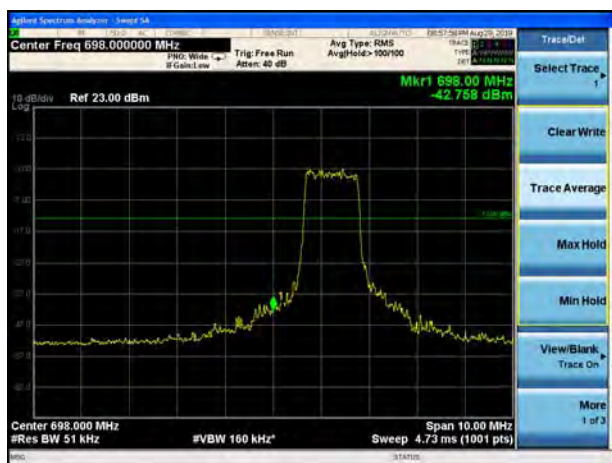
LTE Band 85 16QAM 5MHz CH-Low, 1 RB
