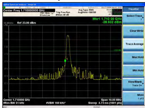
LTE Band 66 16QAM 1.4MHz CH-Low, 100%RB
