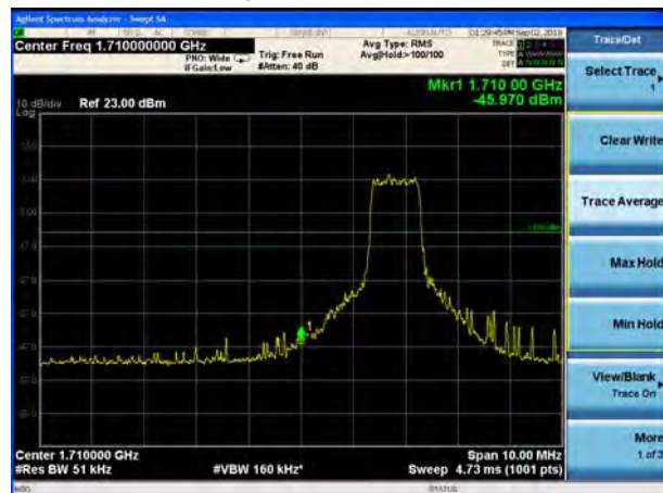
LTE Band 66 16QAM 20MHz CH-Low, 100%RB
