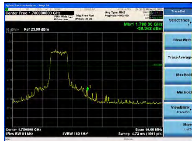
LTE Band 66 QPSK 20MHz CH-High, 100%RB
