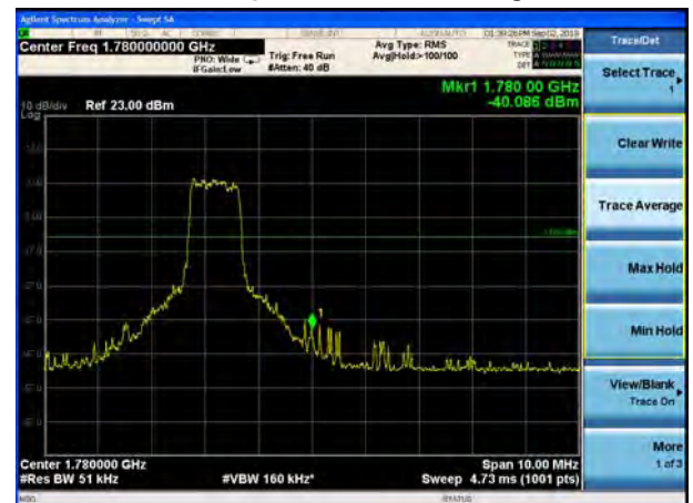
LTE Band 66 16QAM 20MHz CH-High, 100%RB
