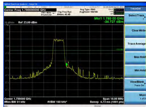
LTE Band 66 16QAM 5MHz CH-High, 100%RB
