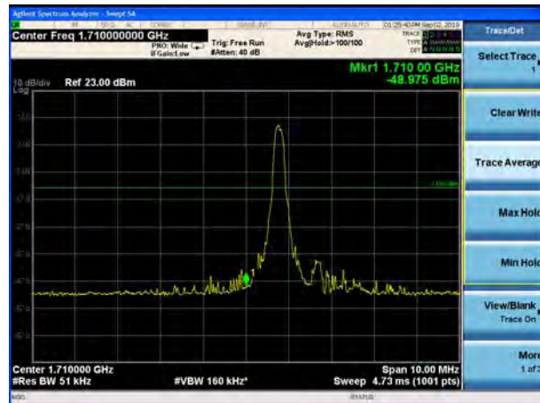
LTE Band 66 16QAM 10MHz CH-Low, 100%RB
