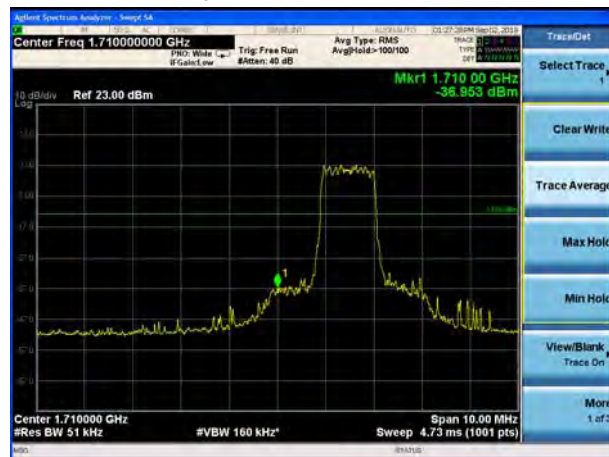
LTE Band 66 QPSK 20MHz CH-Low, 1 RB
