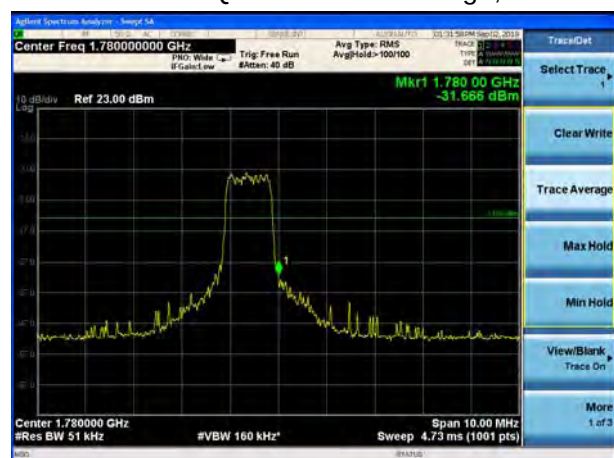
LTE Band 66 16QAM 3MHz CH-High, 1 RB
