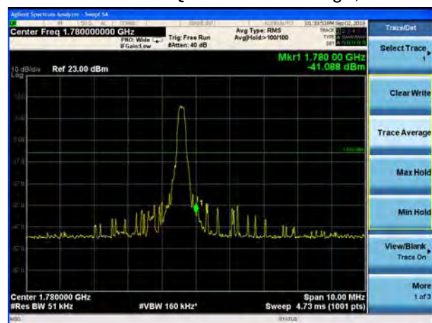
LTE Band 66 16QAM 3MHz CH-High, 1 RB
