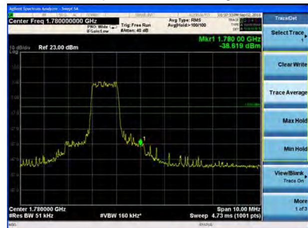
LTE Band 66 QPSK 20MHz CH-High, 1 RB
