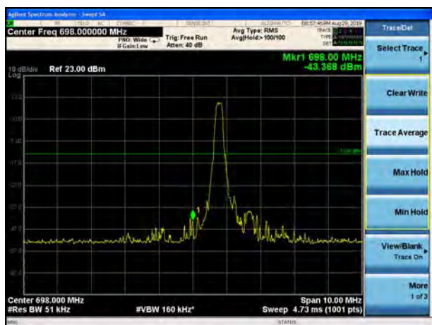
LTE Band 85 QPSK 10MHz CH-Low, 1 RB
