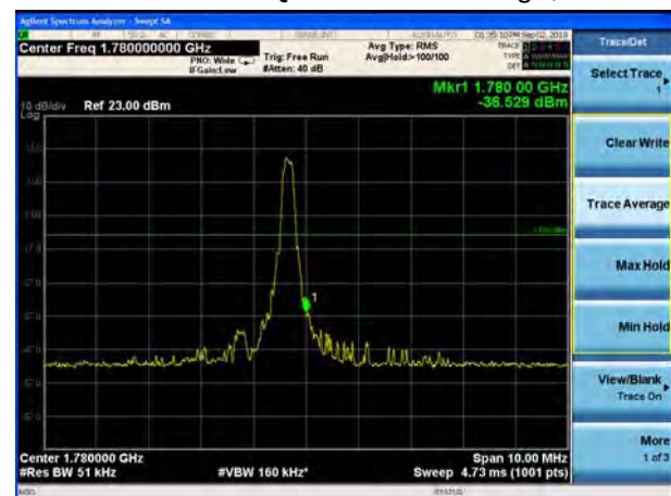
LTE Band 66 16QAM 5MHz CH-High, 100%RB
