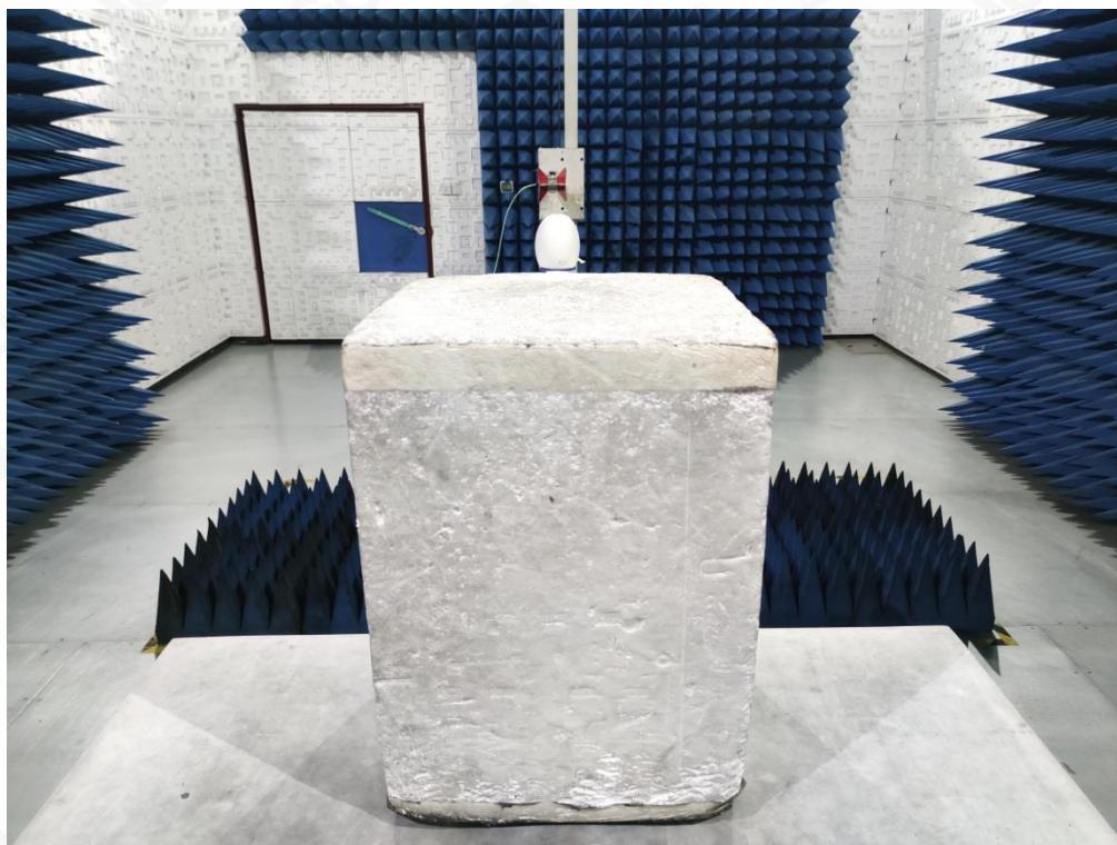
FCC RADIATED EMISSION TEST SETUP ABOVE 1GHZ
