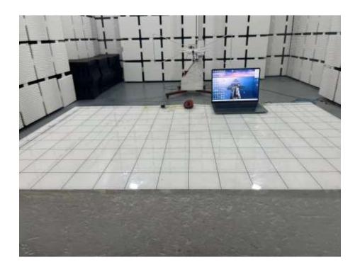
Set-up for Radiated Spurious Emission, Above 1GHz
