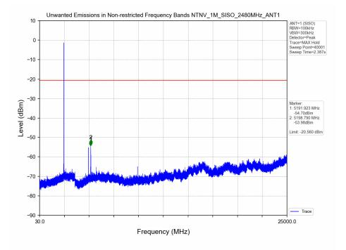
Remark: Cable loss 0.8dB was considered and set in system configuration.
