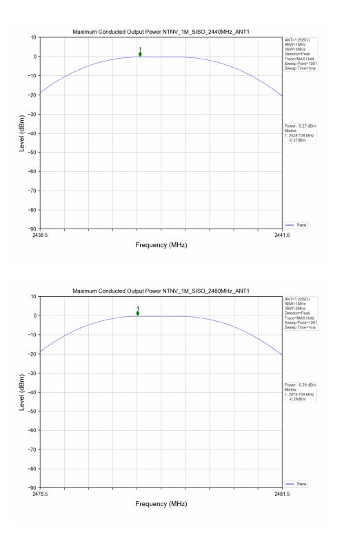
Remark: Cable loss 0.8dB was considered and set in system configuration.
