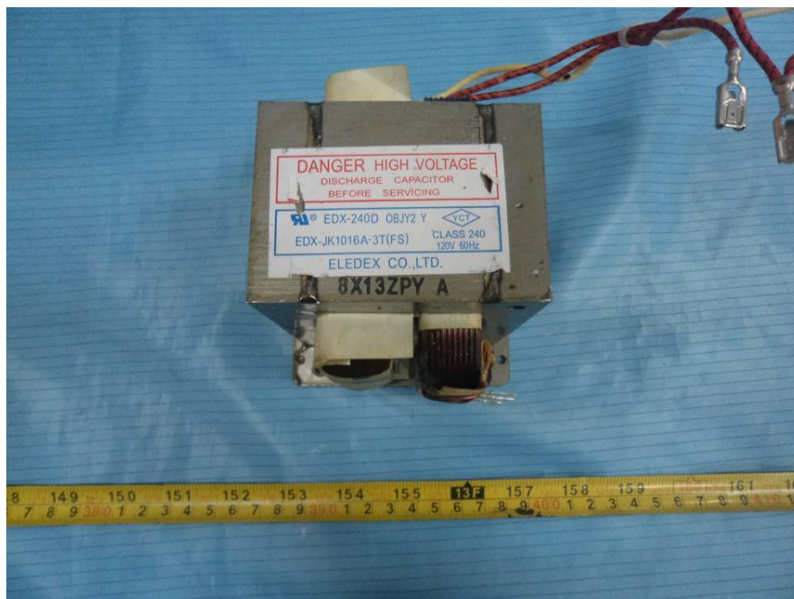
EUT – Power Transformer View
