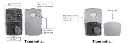
Step 3: Using a small screwdriver match the code to your receiver which was determined in step1.
