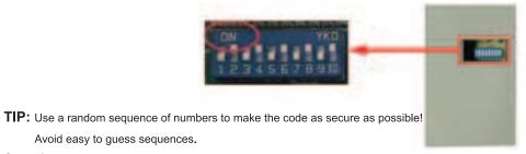
Step 2: Remove the front panel from the transmitter which will expose the 10 digit code selector.
