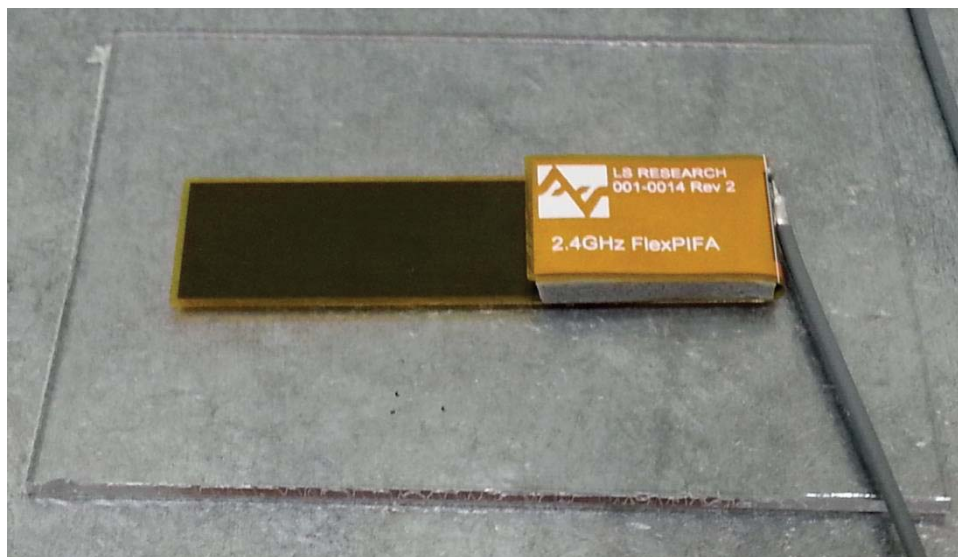
Figure 24 FlexPIFA Mounted on Metal Surface with 1.5mm Thick Polycarbonate Spacer
