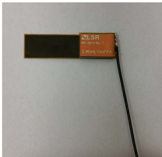
Figure 20 Recommended Cable Routing
