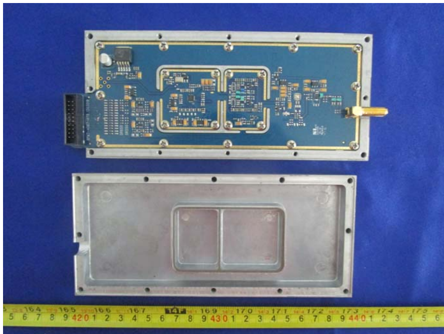
EUT – RX Board Cover Off View
