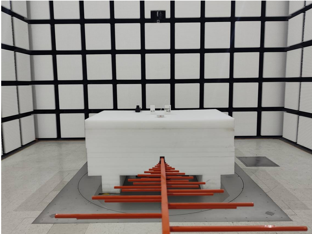
Radiated Emission Below 1GHz View Solar panel
