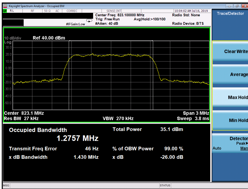
Plot 7-2. Occupied Bandwidth Plot (CDMA BC10 - Ch. 684)
