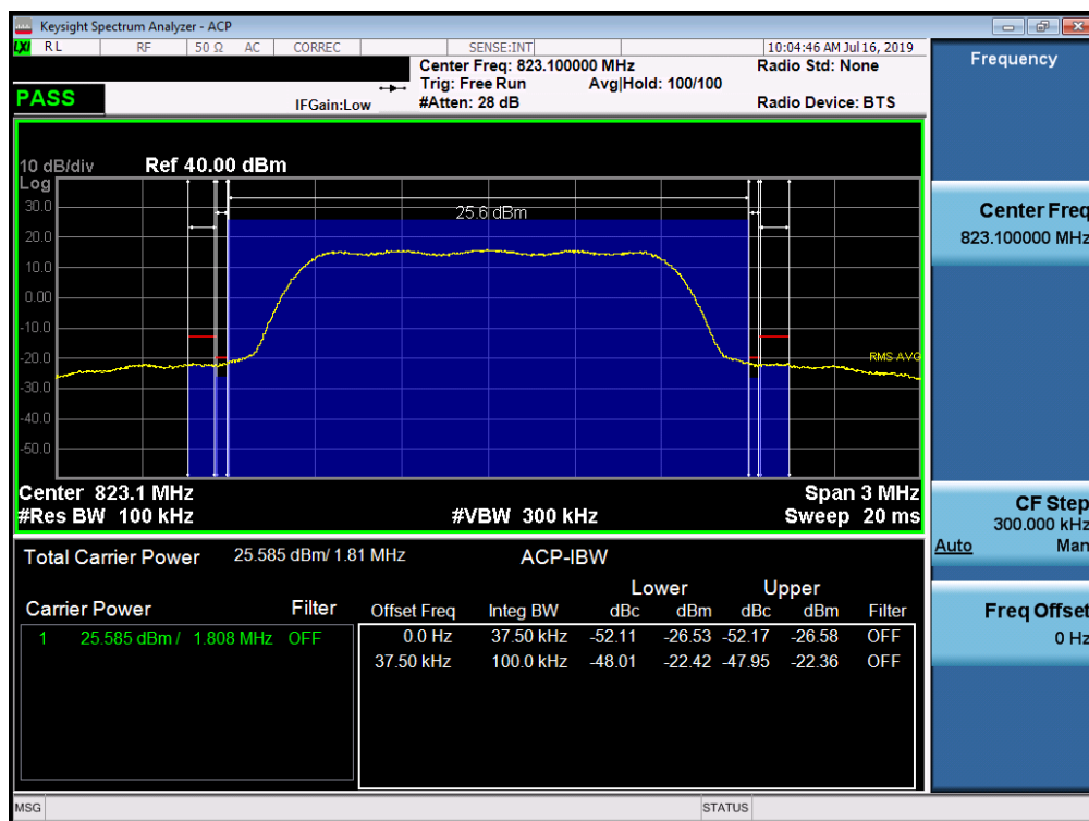
Plot 7-28. Channel Edge Plot (CDMA BC10 - Ch. 684)
