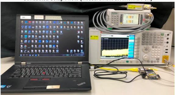
**Conducted Setup Photo (Measurement at Antenna Port)**
