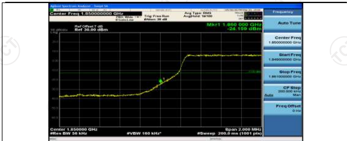
(Channel Bandwidth: 5 MHz)_LCH_QPSK_12RB#6
