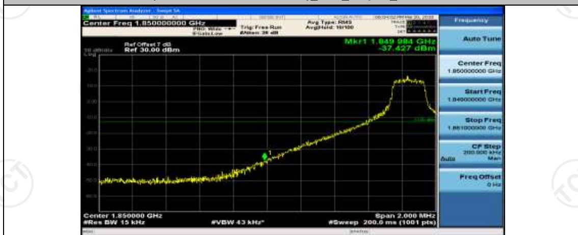
(Channel Bandwidth:15 MHz)_LCH_16QAM_1RB#37
