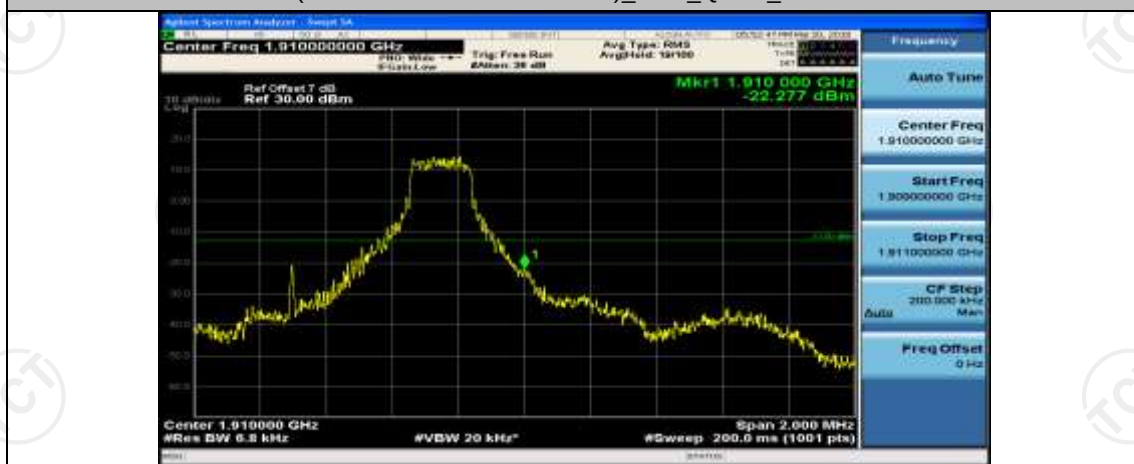
(Channel Bandwidth: 1.4 MHz)_HCH_QPSK_3RB#0
