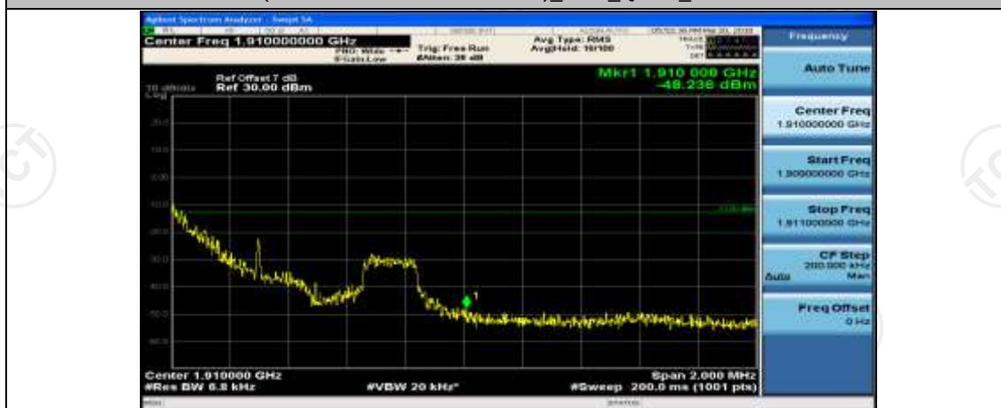
(Channel Bandwidth: 1.4 MHz)_HCH_QPSK_1RB#3
