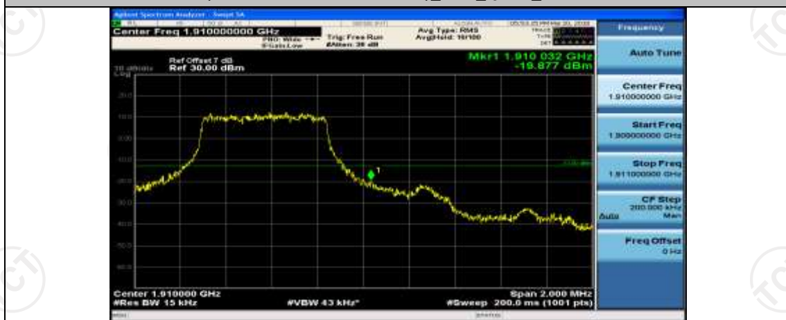
(Channel Bandwidth: 1.4 MHz)_HCH_QPSK_6RB#0
