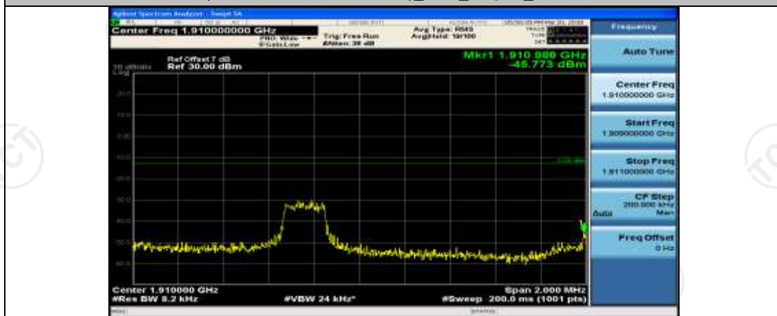
(Channel Bandwidth: 3 MHz)_HCH_16QAM_1RB#7
