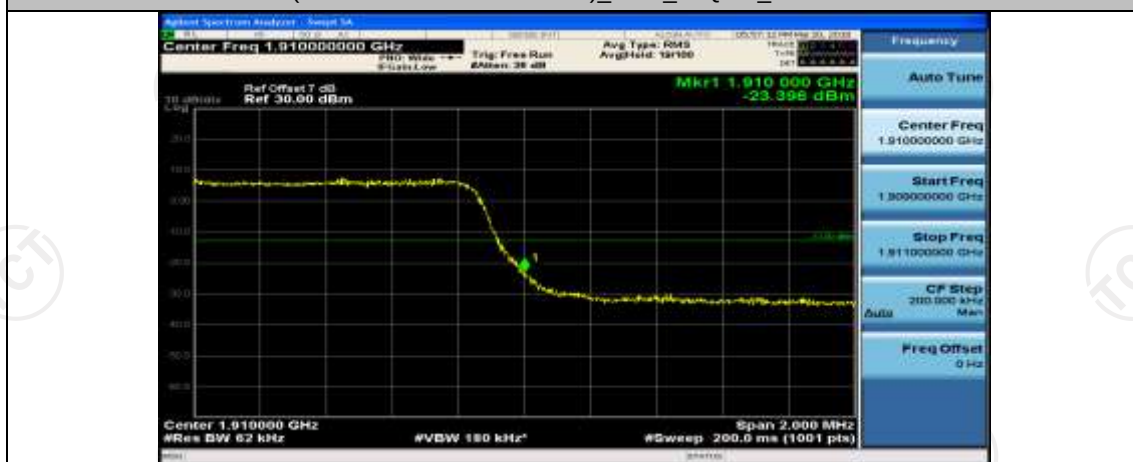
(Channel Bandwidth: 3 MHz)_HCH_16QAM_15RB#0
