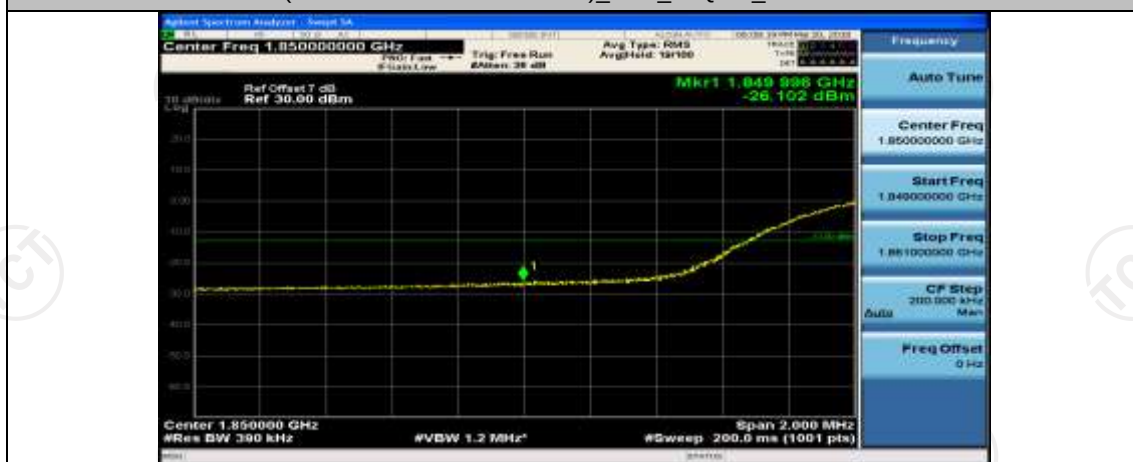
(Channel Bandwidth:20 MHz)_LCH_16QAM_100RB#0
