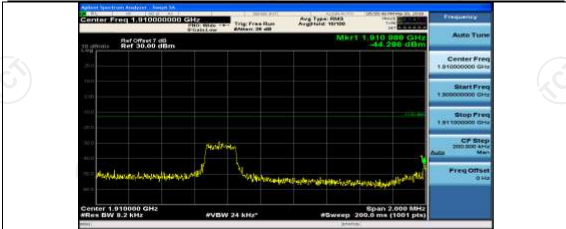
(Channel Bandwidth: 3 MHz)_HCH_QPSK_1RB#7
