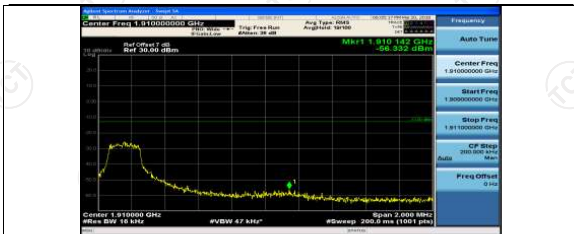
(Channel Bandwidth:15 MHz)_HCH_QPSK_1RB#37
