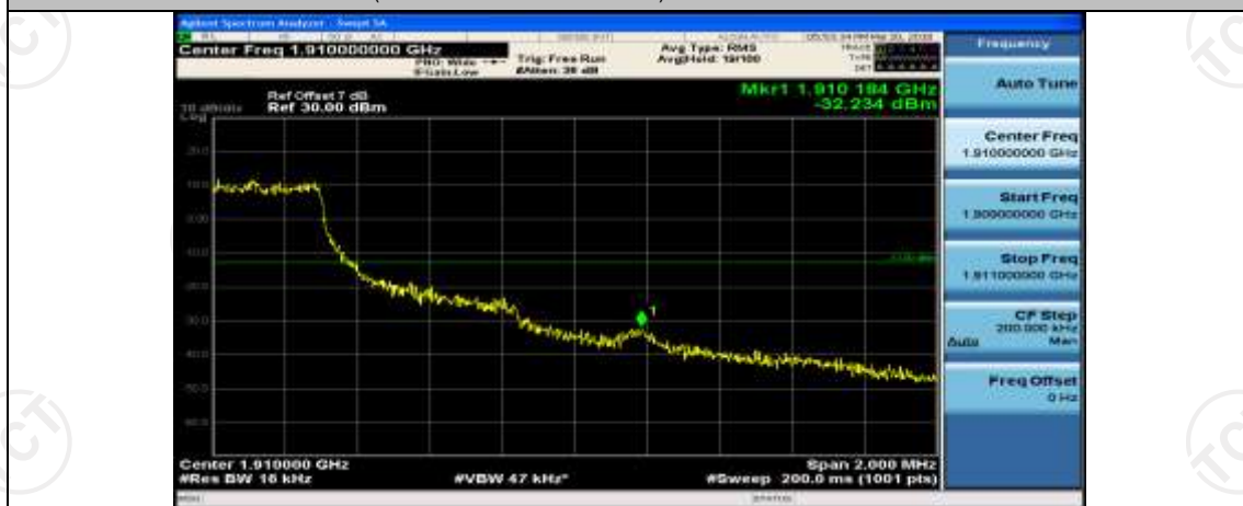
(Channel Bandwidth: 1.4 MHz)_HCH_16QAM_3RB#2
