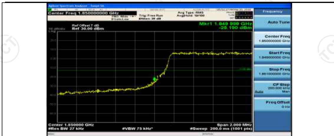
(Channel Bandwidth: 1.4 MHz)_HCH_16QAM_1RB#0
