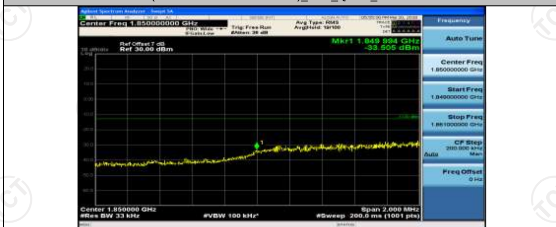
(Channel Bandwidth: 3 MHz)_LCH_QPSK_15RB#0
