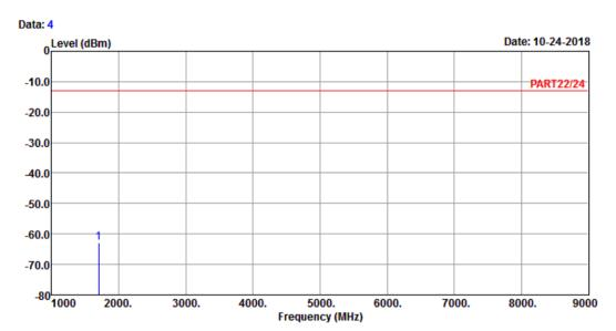
Site : 966 Chamber 5 Condition: PART22/24 VERTICAL Remark : GPRS 850 Link\_H-CH
