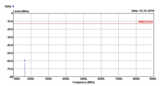
Site : 966 Chamber 5 Condition: PART22/24 VERTICAL Remark : GPRS 850 Link\_L-CH
