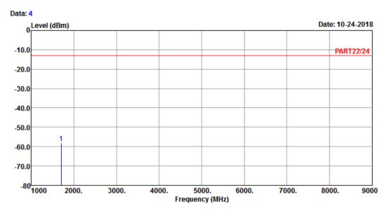
Site : 966 Chamber 5 Condition: PART22/24 VERTICAL Remark : EDGE 850 Link\_H-CH
