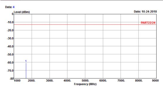
Site : 966 Chamber 5 Condition: PART22/24 VERTICAL Remark : EDGE 850 Link\_M-CH
