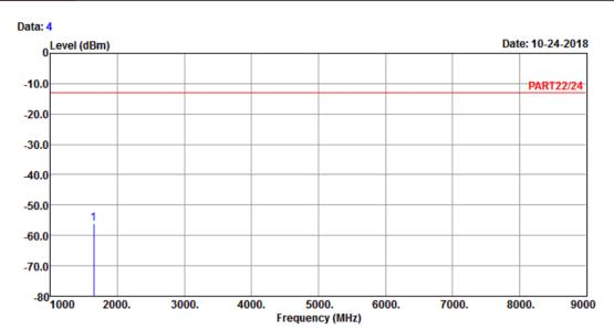
Site : 966 Chamber 5 Condition: PART22/24 VERTICAL Remark : EDGE 850 Link\_L-CH
