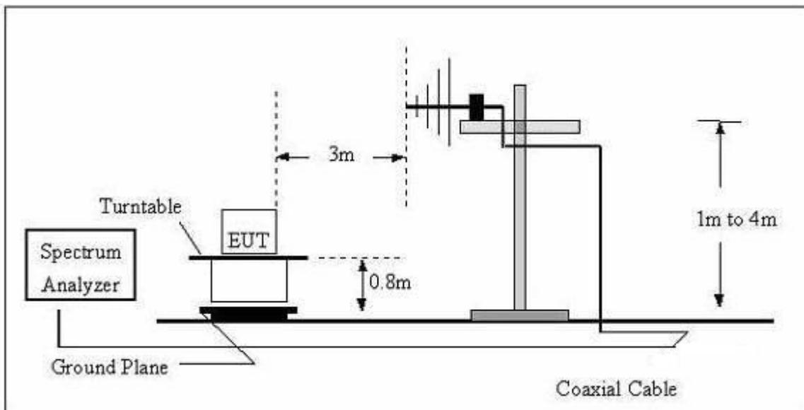
(C) For radiated emissions above 1000MHz
