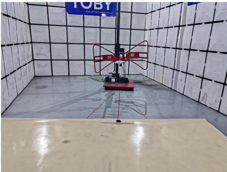
Photo of Setup for Radiated Emission (30MHz~1GHz)
