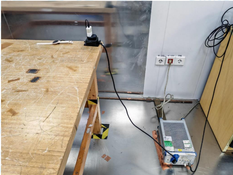
Photo of Setup for Radiated Emission (30MHz~1GHz)
