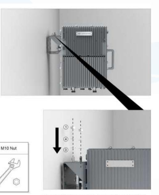
Hang the MP-PS on the mounting bracket  $\,|\,$  and fasten with  $\,2{\times}M10$  nuts.
