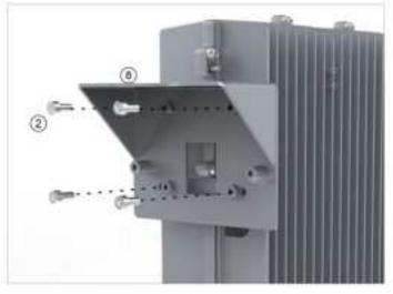
Faster the mounting bracket | to the back of MP-PS with 4×M16×14 screws.
