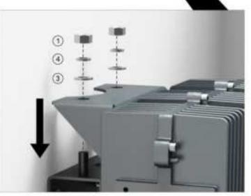
Hang the MP-PS on the mounting bracket  $\,I$  and fasten with  $\,2{\times}M10$  nuts.
