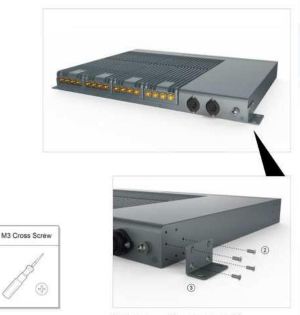
Rotate the hanger 90° and install in AU-PS.
