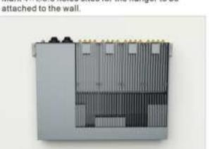
· Drill at the four sites using a percussion drill · Fasten the case with 4×ST4.5 self-tapping screws.
