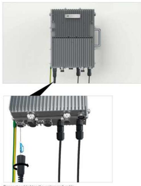
Connect and tighten the waterproof cable (A waterproof sleeve to be purchased separately)to MP-PS.
