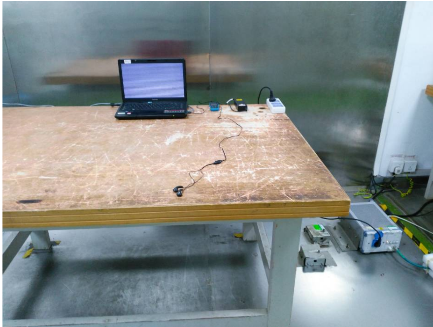
Conducted Emissions - Front View
