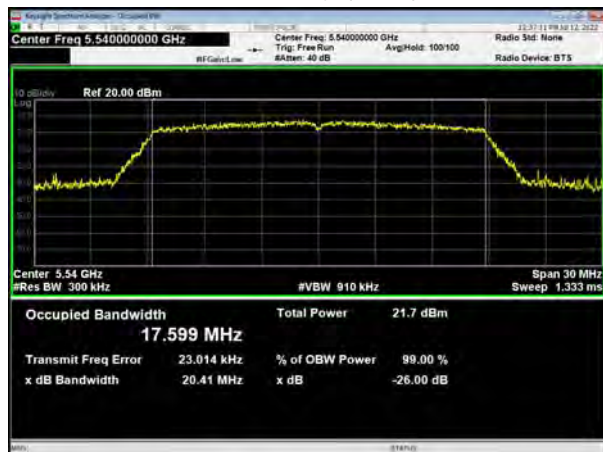
U-NII-2C, 802.11ac VHT20 Carrier frequency (MHz): 5540
