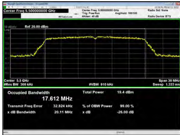
U-NII-2C, 802.11ac VHT20 Carrier frequency (MHz): 5520
