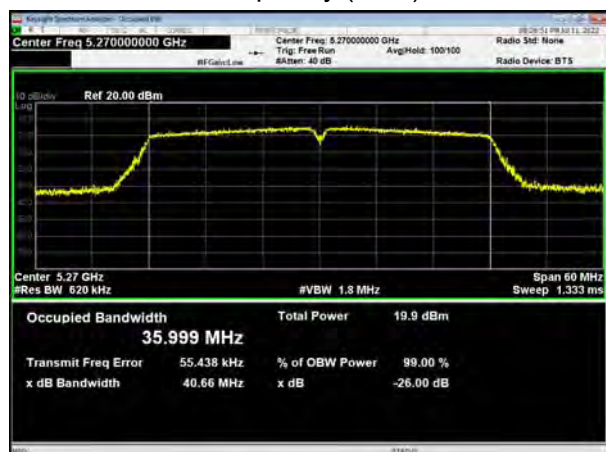
U-NII-2A, 802.11ac VHT40 Carrier frequency (MHz): 5310
