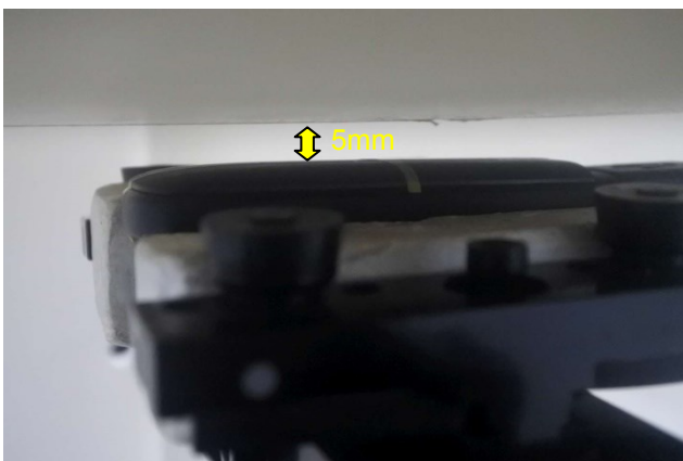
USB Cable Plug-in for USB Configuration 2 (Horizontal Down, Test Separation 5 mm)
