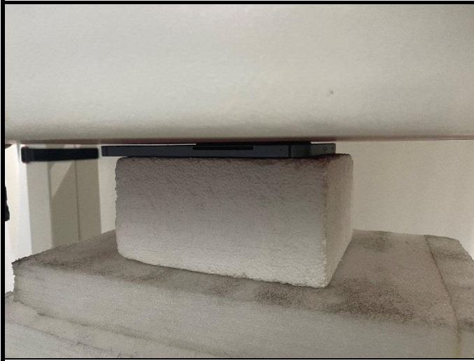
Rear Face of EUT with 0 cm Gap
