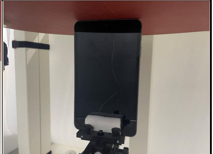
Top Side of EUT with 0 cm Gap
