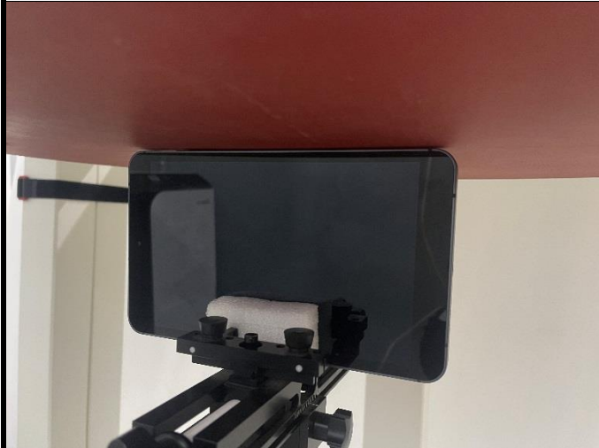
Right Side of EUT with 0 cm Gap
