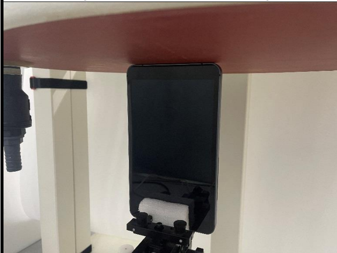
Bottom Side of EUT with 0 cm Gap
