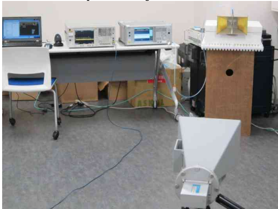
Test Setup for Generating the Radar Waveform
