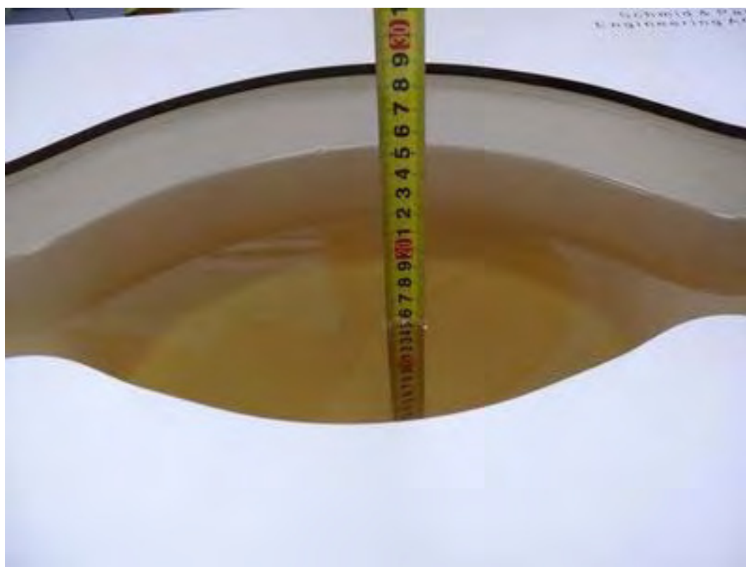
Picture 6: Liquid depth in the flat Phantom (835MHz, 15.4cm depth)
