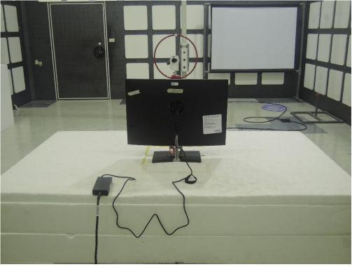
Radiated Emission Set up Photos (Below 1GHz)
