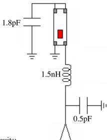
Components used in matching circuits:
