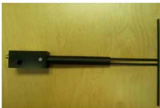
Figure 1 – MVG COMOSAR Validation Dipole
