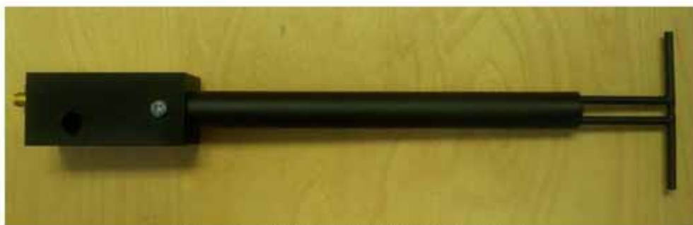
Figure 1 – MVG COMOSAR Validation Dipole
