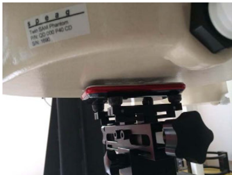
10mm Body-worn Front Side Setup Photo
