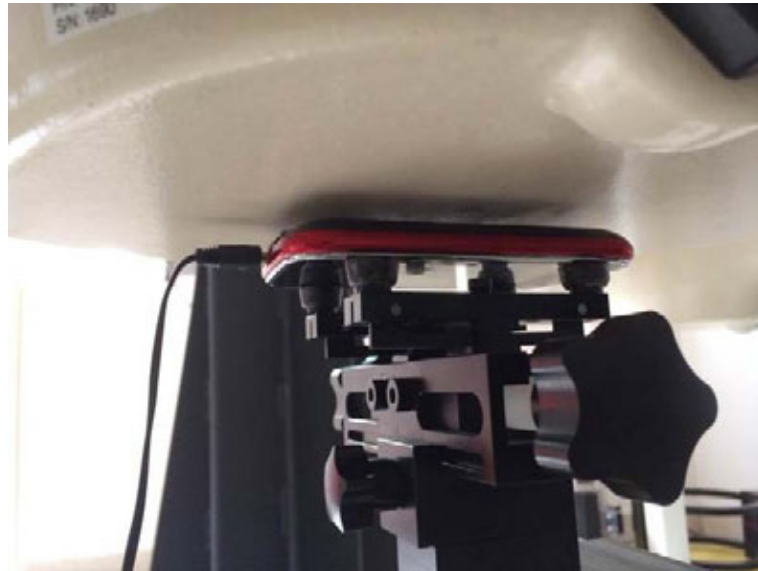
10mm Body-worn Rear Side (With Headset)Setup Photo
