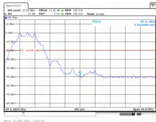
Out Of Band Emission BLE 2M_Channel 39
