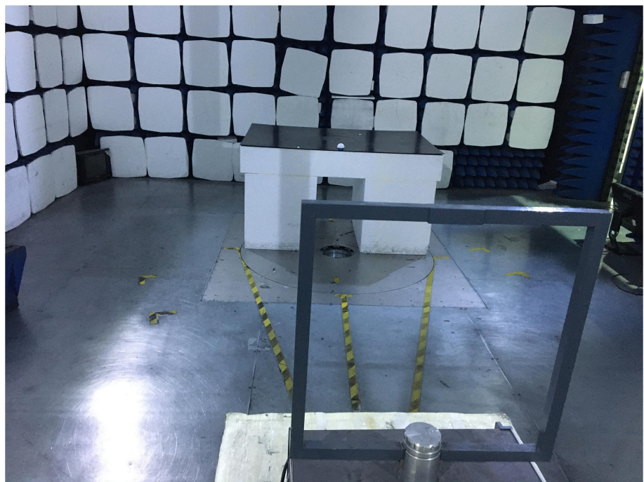
Radiation Emission Test Setup (Below 30MHz)
