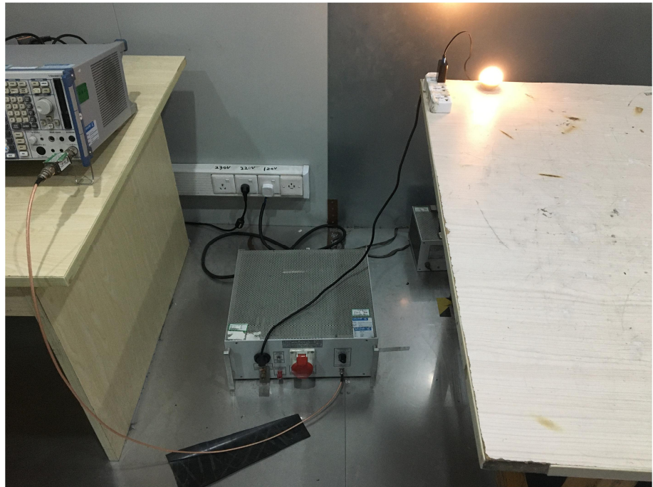
Conducted Emission Test Setup
