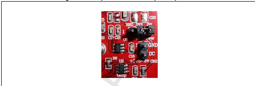
Figure 4. Jumper JP1 set in RF power position
