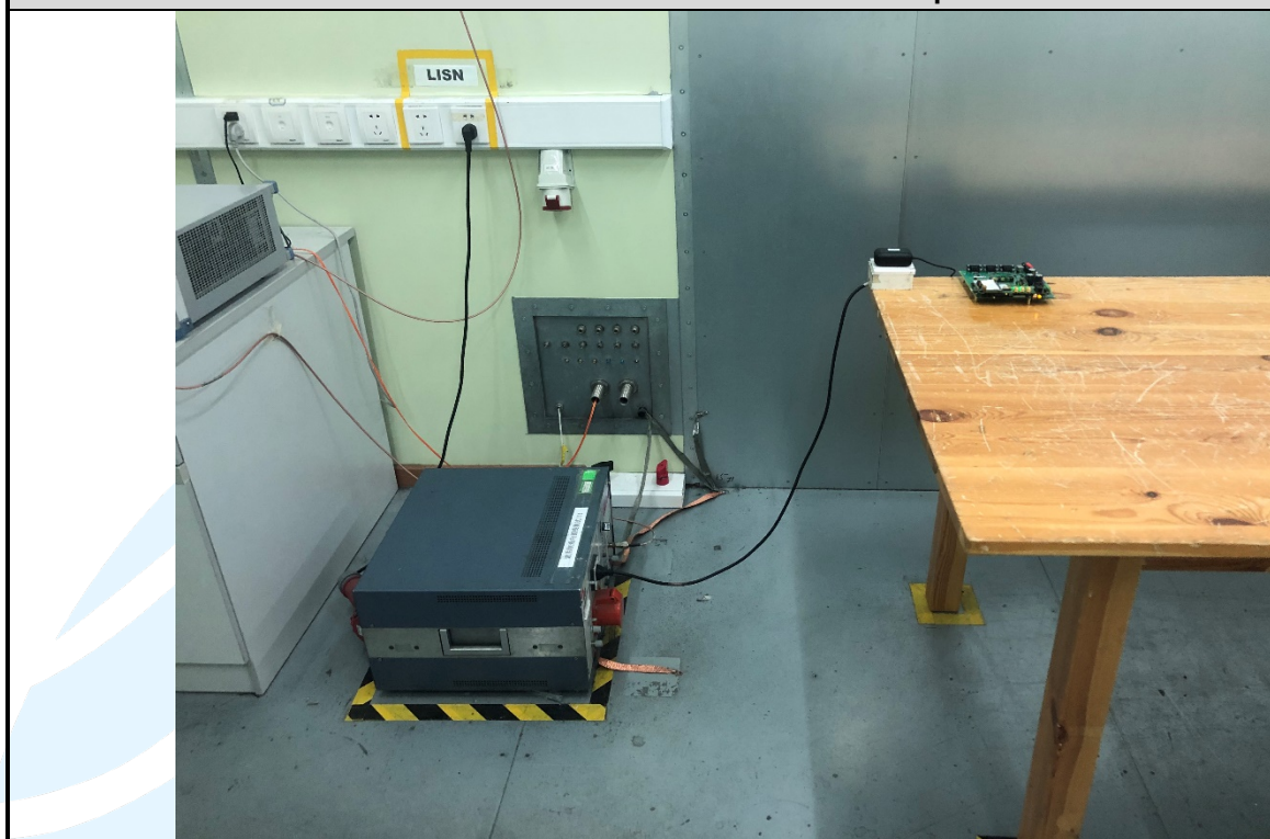
Conducted Emission Test Setup
