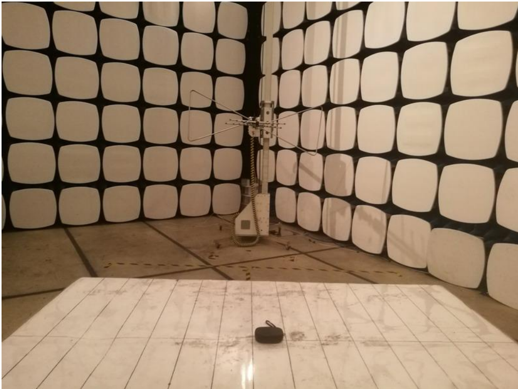
FCC RADIATED EMISSION TEST SETUP
