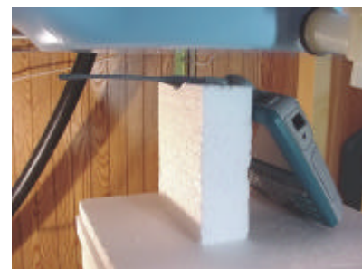
Body SAR Test Setup with 2.0cm separation distance
