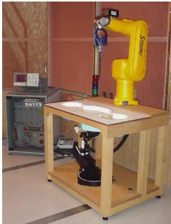
DASY3 SAR Measurement System
