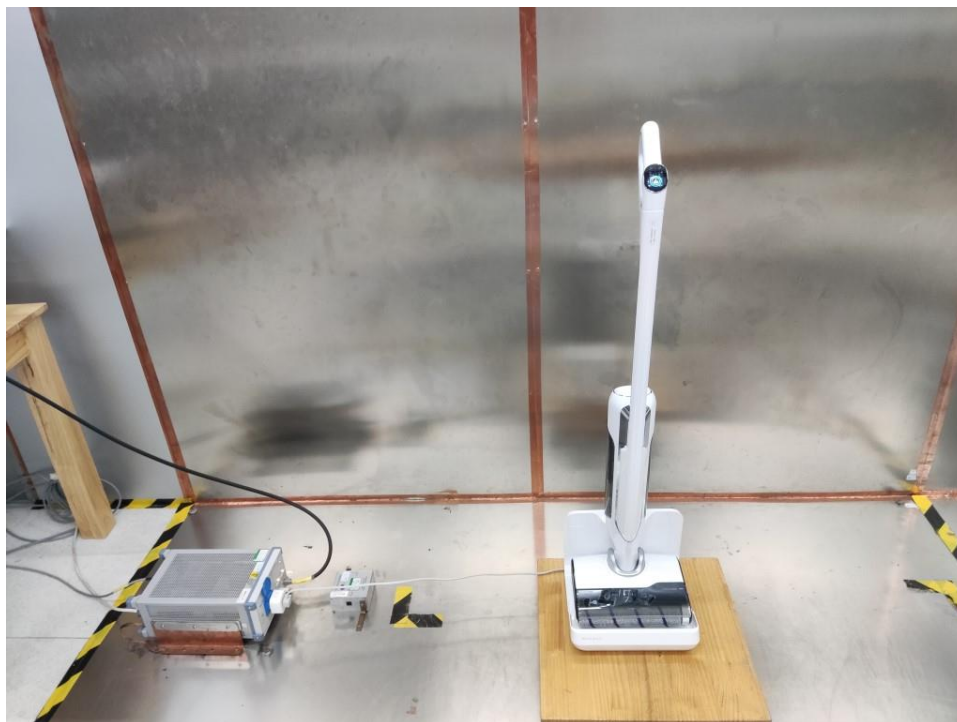
Photograph 3: Set-up for Conducted Emission on AC Mains
