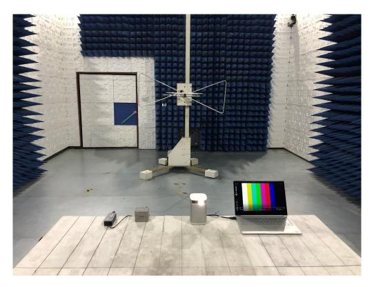
RADIATED EMISSION TEST SETUP ABOVE 1GHZ
