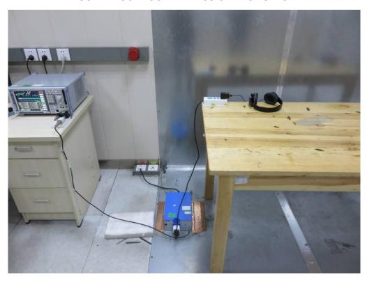
FCC RADIATED EMISSION TEST SETUP
