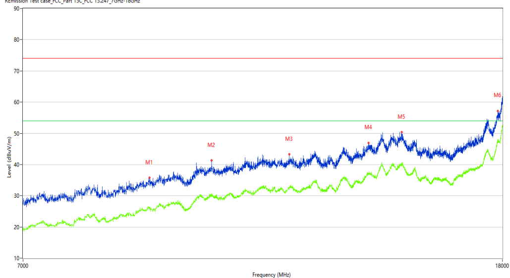
REmission Test case_FCC_Part 15C_FCC 15.247_7GHz-18GHz
